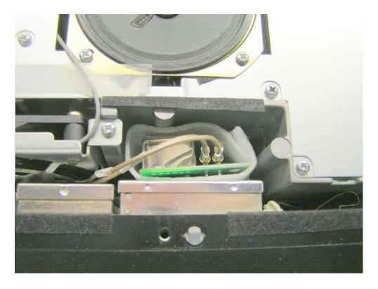
Figure 6. Locating the B+ and Ground connections on the Main Unit.
